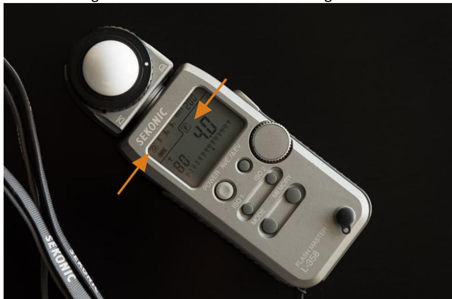
*A light meter set to measure ambient light. The F refers to the f-stop and the T is the shutter speed. I set the ISO to 200 (see top right) and the aperture to f4. I then measured the light and was given a shutter speed of 1/80.*
