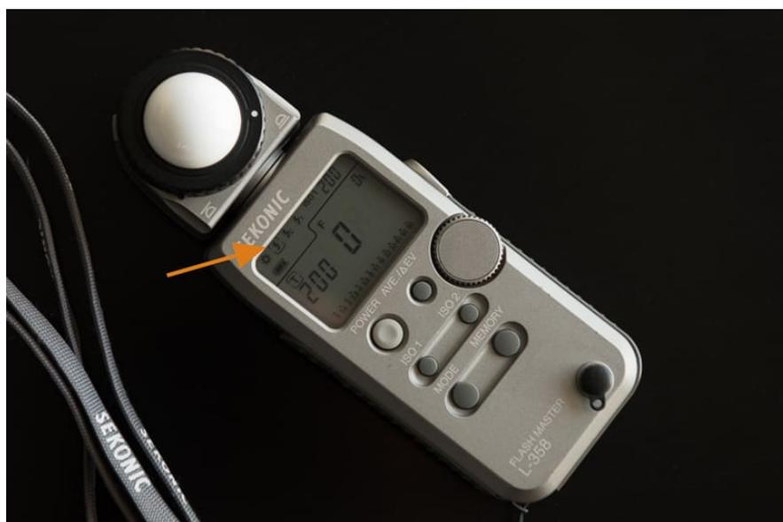
*The light meter is set to measure flash. The ISO is set to 200 and the shutter speed is set to 200. When the flash triggers the light meter will measure the light and give me a reading of the f-stop, which is currently set to 0.*
