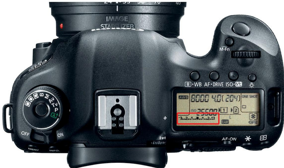
Depending on the camera, you may get a graphical representation of the light meter's reading. Many cameras show a scale in the viewfinder and/or on the LCD top or rear screens that shows if the current aperture and shutter speed settings will over- or underexpose the image. You can use this information to make an informed decision to alter the exposure of the image from the baseline meter reading. The scale generally has hash marks that indicate stops of exposure.
